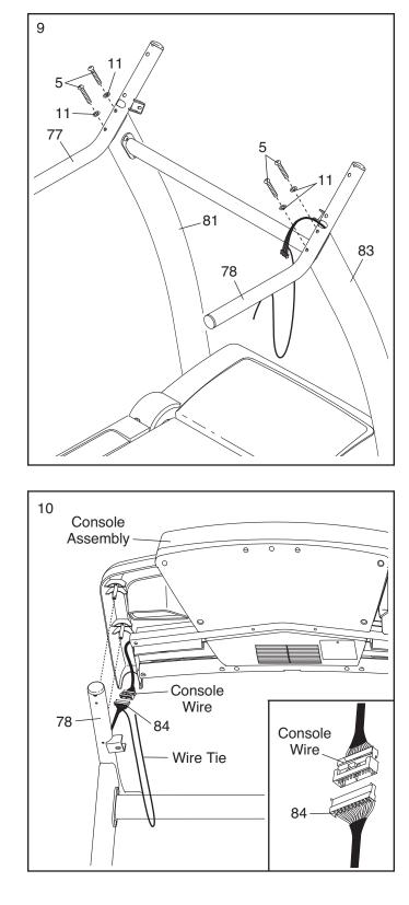
10. Have a second person hold the console assembly near the Right Handrail (78). Connect the Wire Harness (84) to the console wire. See the inset drawing. The connectors should slide together easily and snap into place. If they do not, turn one connector and try again. IF THE CONNECTORS ARE NOT CONNECTED PROPERLY, THE CONSOLE MAY BE DAMAGED WHEN YOU TURN ON THE POWER. Next, remove the wire tie from the Wire Harness. Insert the connectors and the excess wire into the Right Handrail.
